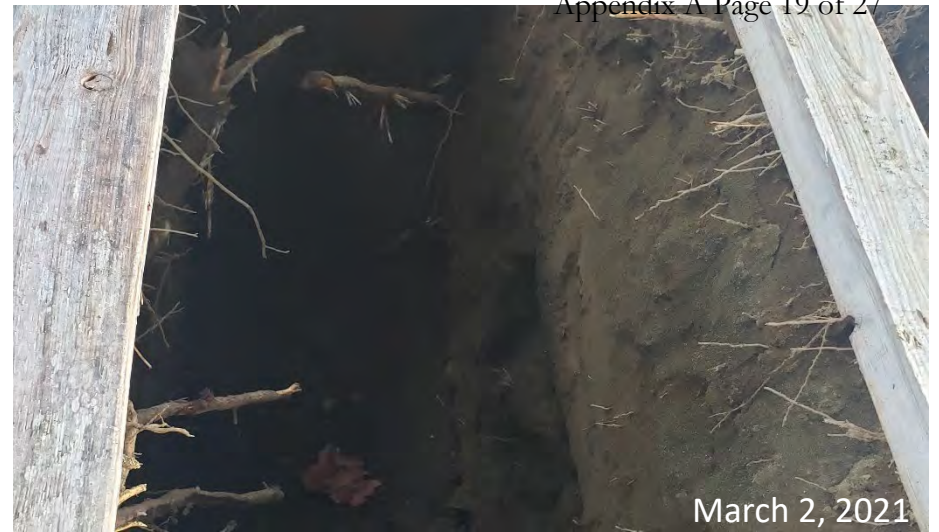
Photo 12 – Sandy fluvial deposits noted in test pit with roots and rootlets.
